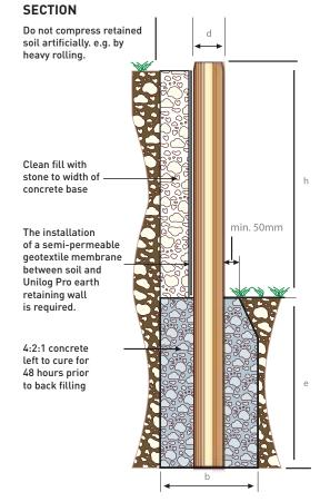
Bottom of trench to be cut clean, level and undisturbed. A free draining levelling bed should be provided.
